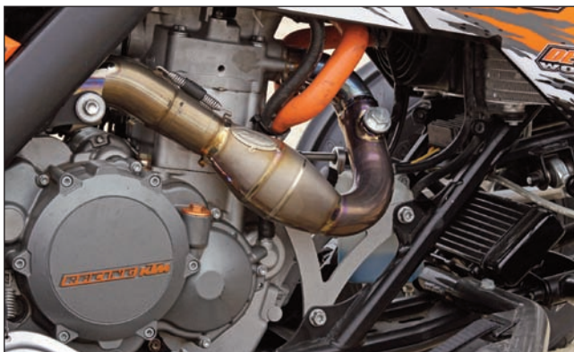
The FMF MegaBomb head pipe has an O2 sensor bung in it to fine-tune the jetting with a wide-band sensor. It makes great power without being overly loud.
